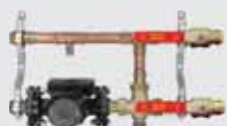
Mixing station Base unit - For supply temperature modulation - Equipped with circulator Model 2801.1US, 2801.9US Components Isolation ball valves, mounting bracket, supply temperature sensor well, 3-speed circulator Model 2801.0US
